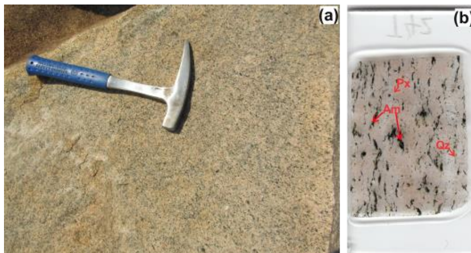
Figure 5. Field photo and scanning image of amphibole granitic gneiss (X= 437,341; Y= 617,910) (m) (a) Outcrop of the amphibole granitic gneiss (b) Scanning image of the amphibole granitic gneiss Qz : quartz, Am : amphibole, Px : pyroxene.
